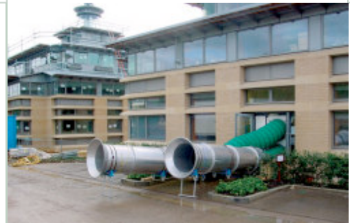
Air-barrier specifications and testing are required in Great Britain, where this blower-door test is taking place at a new commercial building. Large blower doors like these depressurize a building, allowing air-leakage testing.
