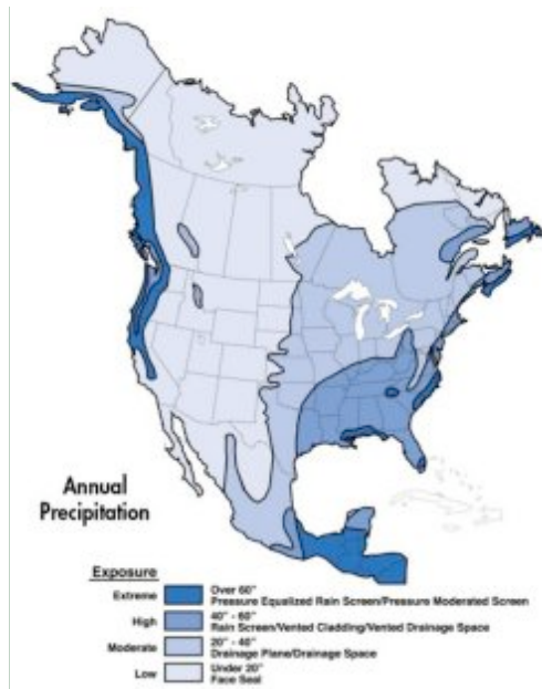
North America divided into four zones based on annual precipitation, with suggested cladding system approach for each zone.
